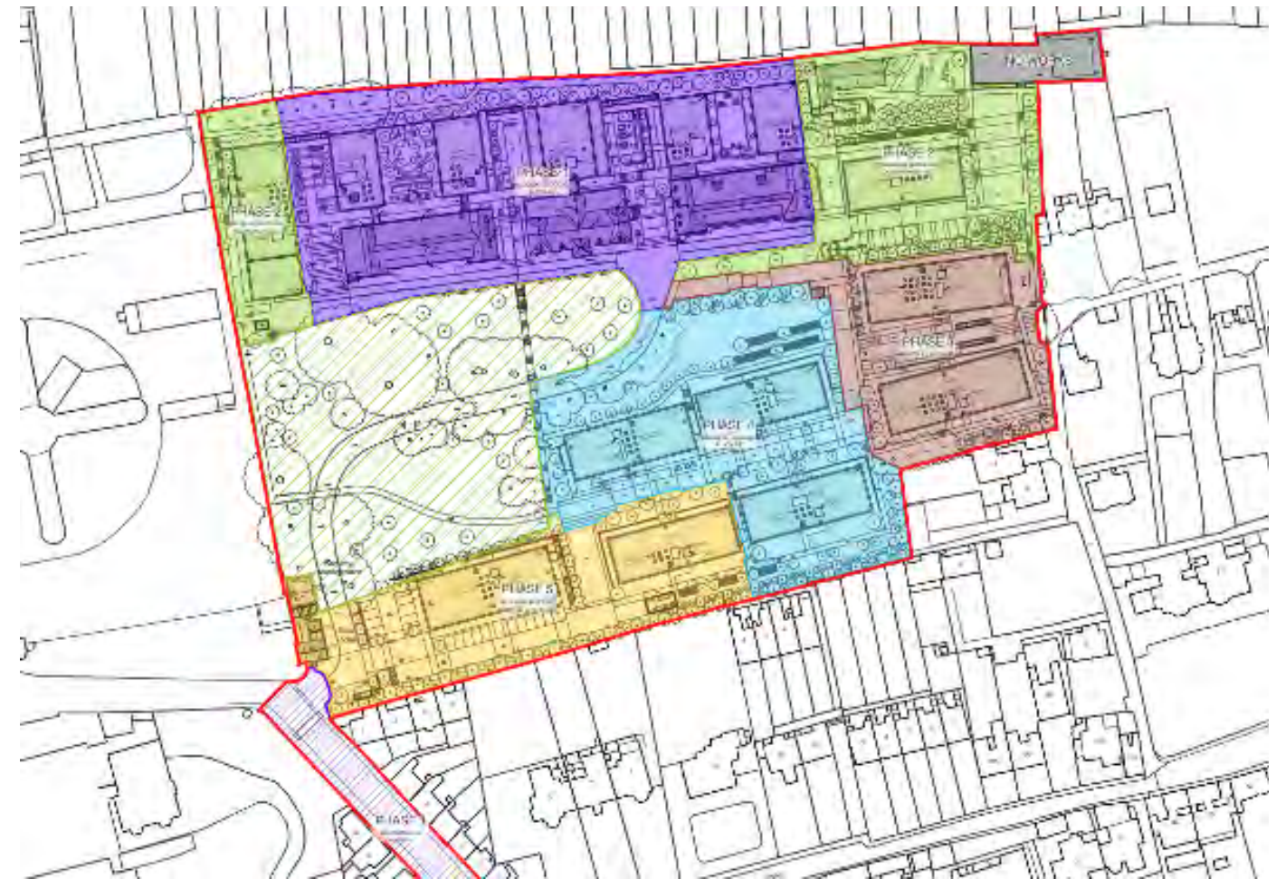
Figure 2.9 Construction Phasing Plan
